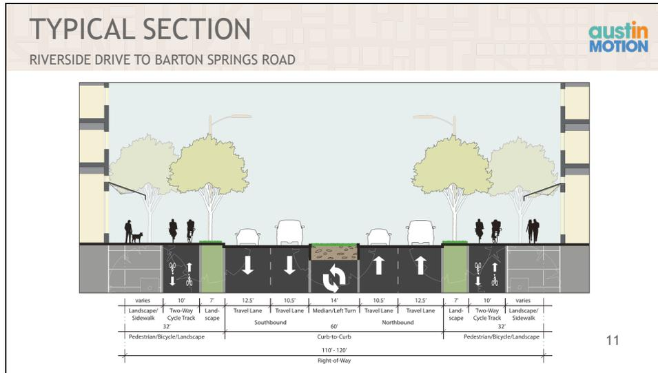
This slide shows the proposed typical cross-section for South Lamar Boulevard between Riverside Drive and Barton Springs Road. These improvements reflect the ultimate vision for the South Lamar corridor, and are funded for construction.
