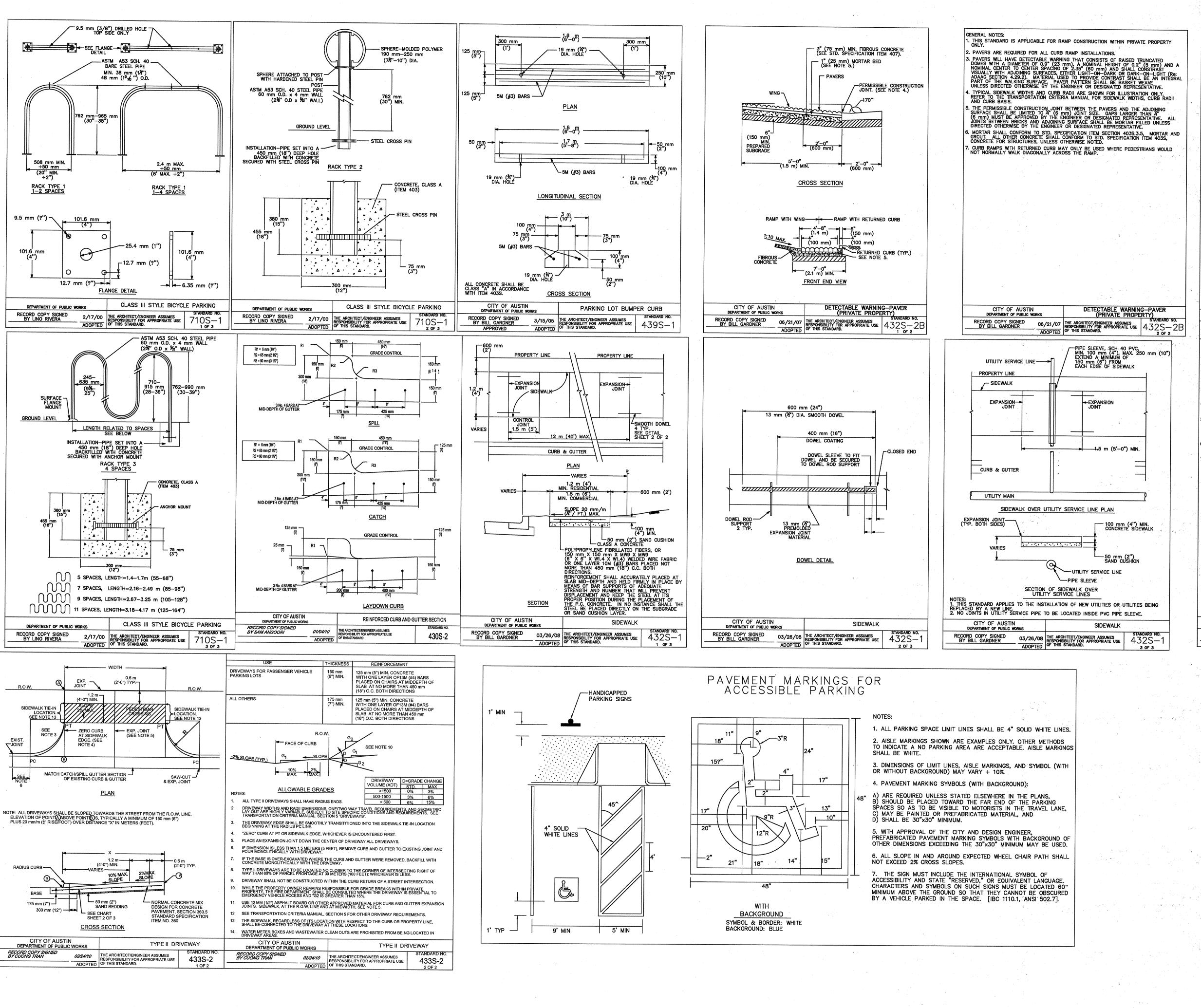
3" (75 mm) MIN. FIBROUS CONCRETE (SEE STD. SPECIFICATION ITEM 407). 1" (25 mm) MORTAR BED (SEE NOTE 5.) -PERMISSIBLE CONSTRUCTION JOINT. (SEE NOTE 4.) the same of the sa (150 mm) MIN. PREPARED SUBGRADE 4'-8" 6" (1.4 m) (15 4" (100 mm) (100 mm) RETURNED CURB (TYP.)
