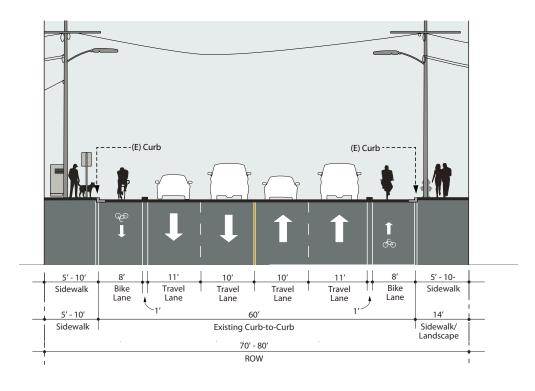
**Interim Option 3:** This is a less intensive intervention, with separated cycle tracks within the existing 60-foot roadway. This could only occur where the center turn lane is eliminated.
