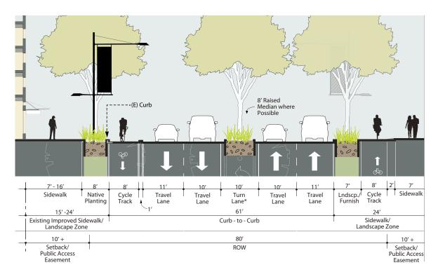
**Hybrid of Option 1 & 2:** This is a hybrid of the two ideal sections that could be employed along recently completed streetscapes like the Post or Gibson. A separated cycle track could be introduced along the completed streetscape with a "behind the curb" cycle track on the opposite side.
