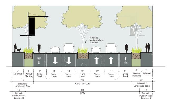
**Idealized Option 2:** This is a variation where the cycle track is located within the roadway with a 12" barrier separating it from the auto lanes. Like Option1, it would require a building setback and public access easement on the many portions of the corridor with less than 100' of ROW.
